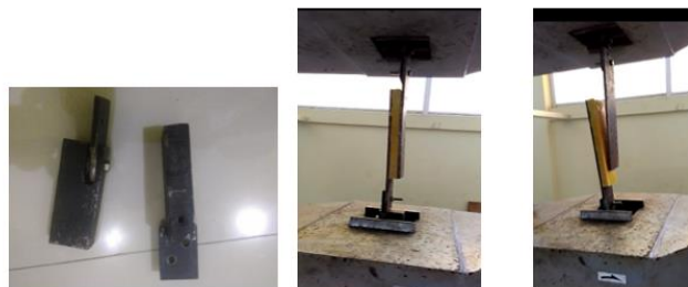
Gambar 8 Uji geser Sandwich Panel
