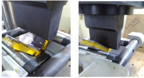
Gambar 9 Uji lentur Sandwich Panel
