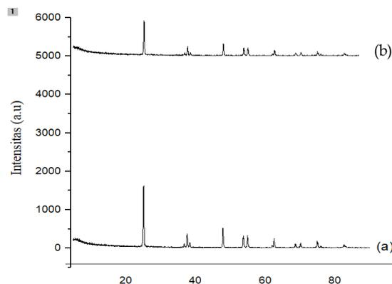
**Gambar 2.** Pola difraktogram (a) TiO<sub>2</sub>, (b) TiO<sub>2</sub>/AgNPs (1)
