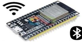
Gambar 2.4 ESP-32 Development Board 38 Pin
