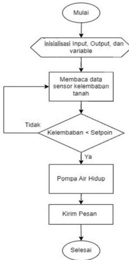
Gambar 4. Diagram alir Receiver
