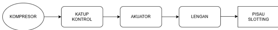
Gambar 4: Flow chart prinsip kerja alat pembersih meja mesin computer numerical control (CNC) laser cutting
