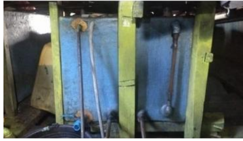
Gambar 2: Tangki bahan bakar KM Binama No.7
