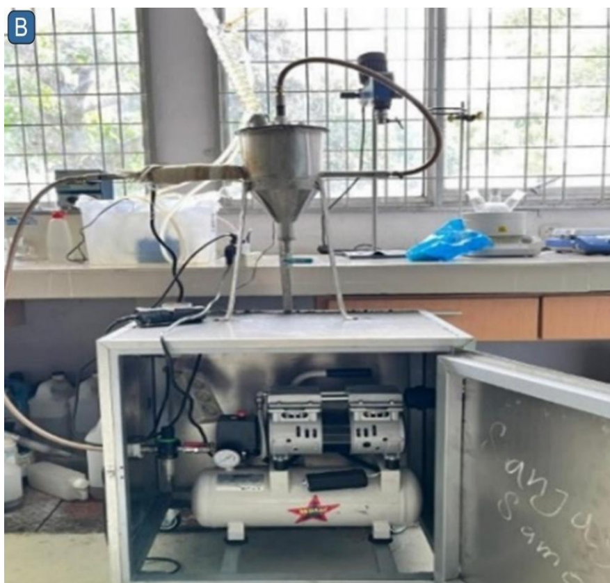
Figure 4. Completed biodiesel production plant
