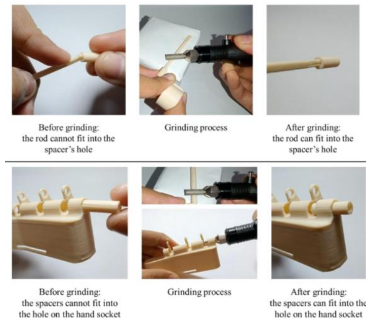
Figure 8. The Grinding Process
