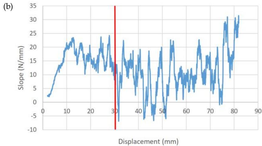
Figure 7 (b) Slope vs. Displacement Curve of *Sus* Cake
