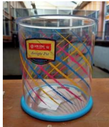
Figure 2 Acrylic Container Used as Specimen Holder for Multi-Sample Compression
