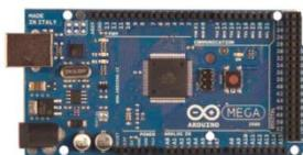
Gambar 4. Arduino Mega 2560
