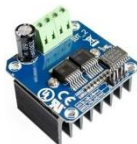
Gambar 4. Motor Driver BTS 7960 Sumber: Waskita Adijarto., 2021
