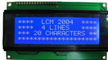
Gambar 2. LCD 20x4
