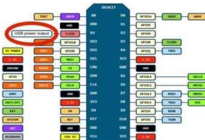
Gambar 1 Mapping Pin NodeMCU V3 Sumber: Silitonga,2019
