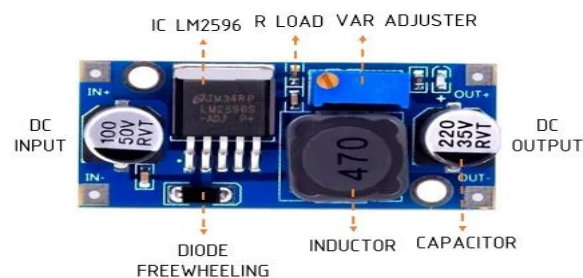
Gambar 4. Modul Stepdown LM2596 Sumber: Riyan, dkk, 2019
