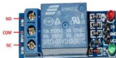
Gambar 3. Relay 1 channel Sumber: Akbar Abadi, 2020
