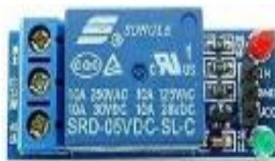
Gambar 3. Relay 1 channel
