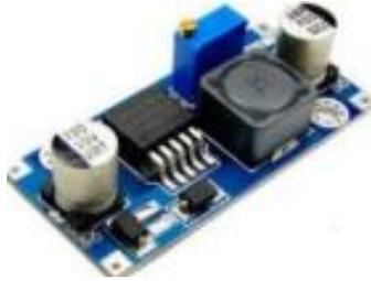
Gambar 4. Modul *step down* LM2596
