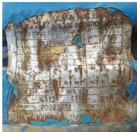
**Gambar 2. Name Plate Motor 45 kW**
