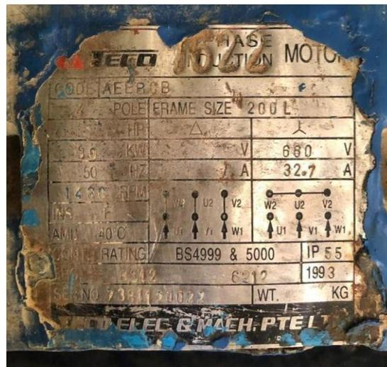
**Gambar 1. Name Plate Motor 30 kW**
