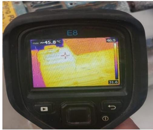
**Gambar 8. Pengecekan Temperature Body Motor 45kW**
