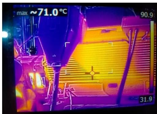
**Gambar 7. Pengecekan High Temperature Body Motor 30kW**
