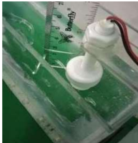
Figure 5 Sensor State When Detecting Water
