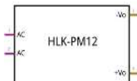
Fig 7. 22V to 12V Adapter Circuit
