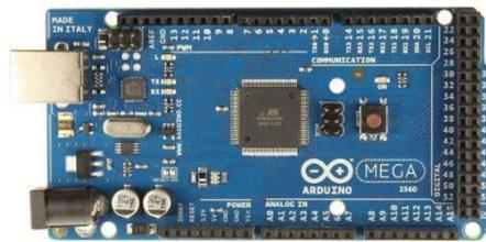
Gambar 1. Arduino Mega 2560
