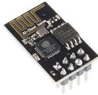
Gambar 6. ESP8266 (ESP-01)
