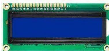
Gambar 2. LCD 16 x 2 I2C
