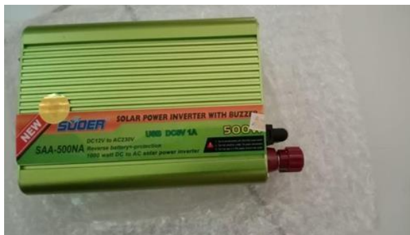
Gambar 5. Inverter 500 W (The Specialist Panel Surya 2022)
